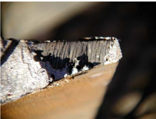
Figure 5. Total lack of fusion at rail foot due to mould misalignment
