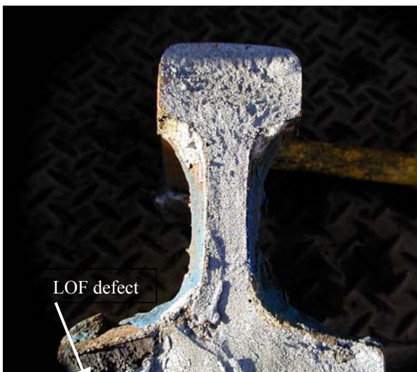
Figure 4 Lack of fusion in the rail foot
