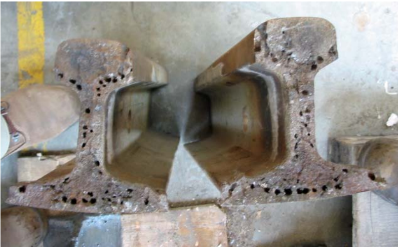
Figure 7. Gross porosity in the weld
