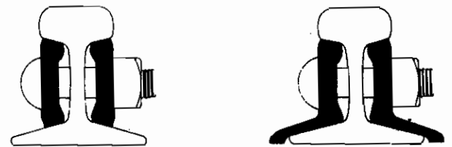
Splice (Flat) Bar Angle Bar Planchuela Plana Planchuela Angular
