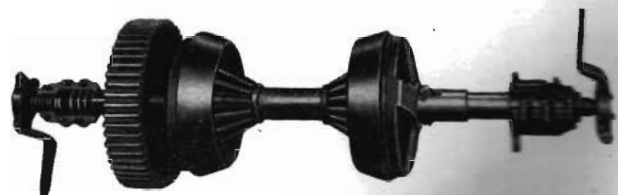
Swing Shaft with "T" Type Clutches and Renewable "Orcoin" Friction Blocks. (Shows friction screw with ballnut removed.)
