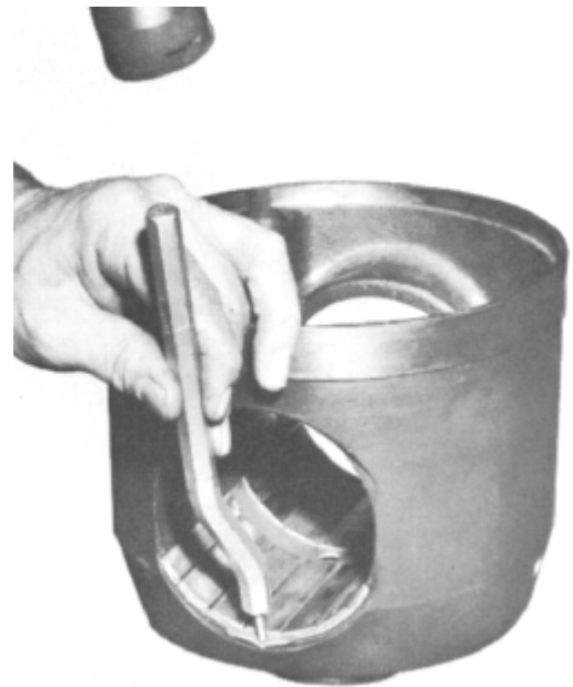
Fig. 5-15 -- Piston Pin Bearing Insert Installation
