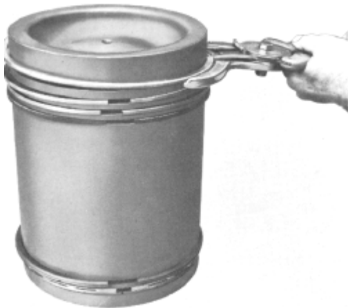
Fig. 5-14 - Installation Of Top Compression Ring
