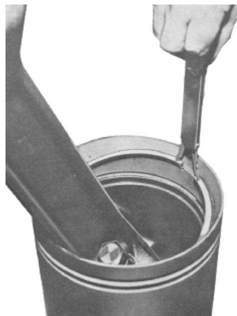
Fig. 5-17 - Installing Piston Snap Ring
