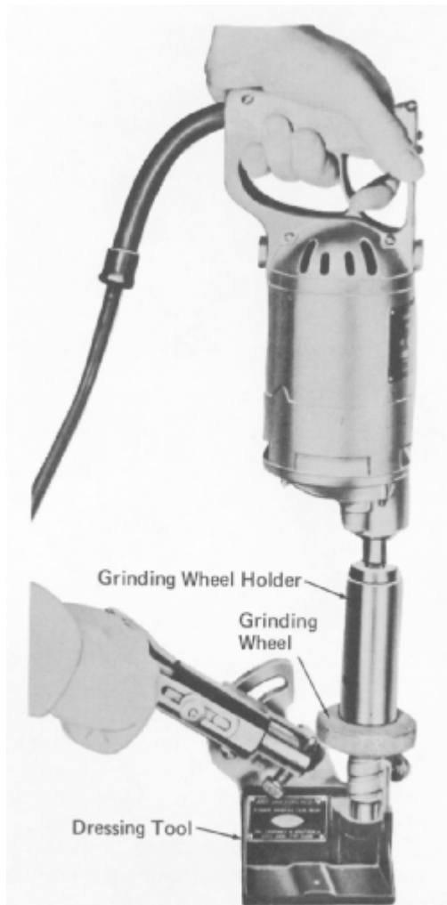
Fig. 2-10 - Dressing Valve Seat Grinding Wheel
