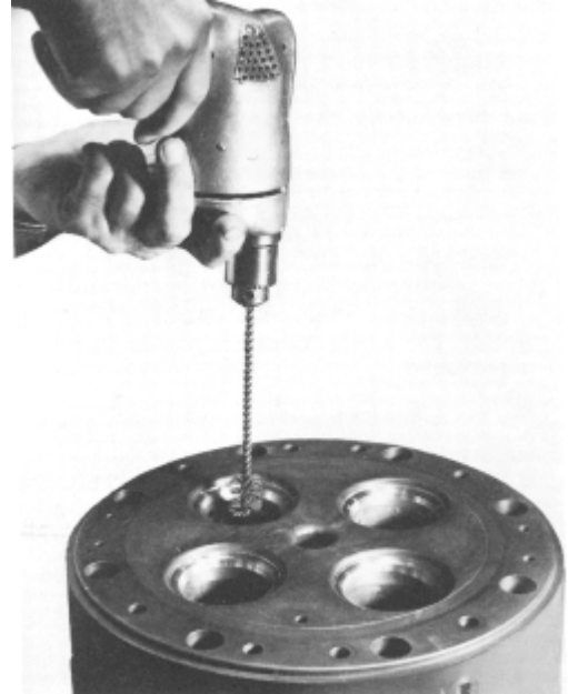
Fig. 2-5 - Cleaning Valve Guides
