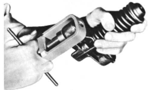
Fig. 2-28 - Installing Lash Adjuster
