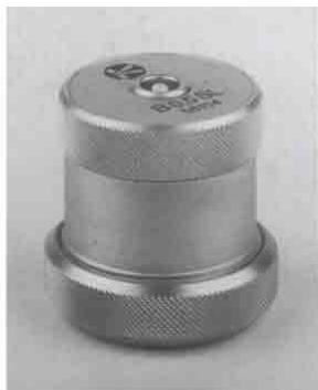
Probe B0.5SL, identical in shape to coarse grain probes K0.5S and K1S.
