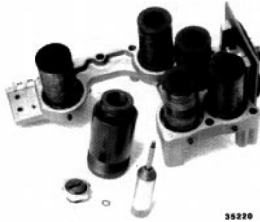
Figure 5. Receiver Assembly with New Coils Attached
