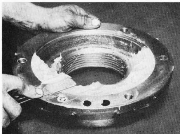
Fig. 5 - Roughly Formed Grease Contour
