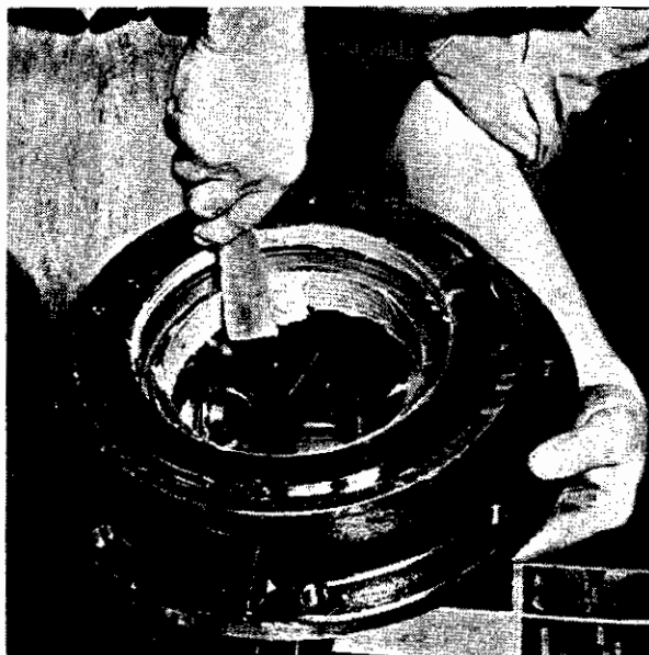
Fig. 3 - Grease Application To Labyrinth Grooves
