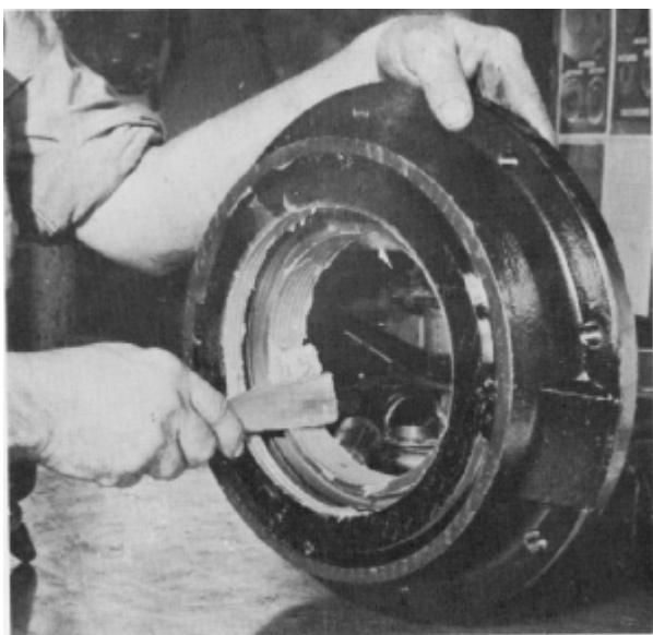
Fig. 2 - Grease Application To Labyrinth Grooves
