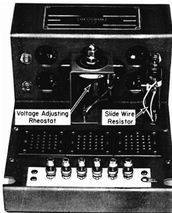
Fig. 2 - Operator Unit And Regulator Chassis
