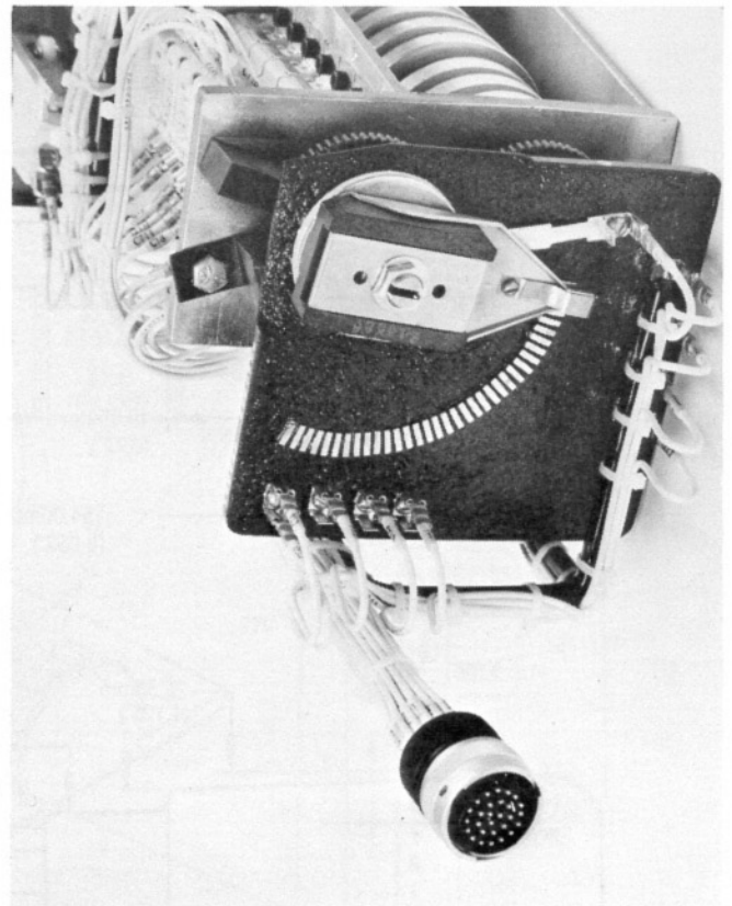
Fig. 8 - Dynamic Brake Rheostat With Wiring Harness connections which enable proper interface with the cam drum and at the side of the housing to interface with the reverse cam.
