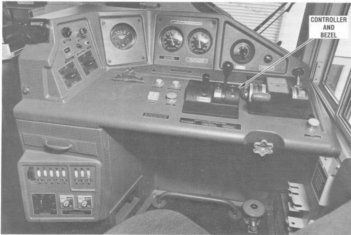
Fig. 3 - Manual Dynamic Braking Equipped Control Console
