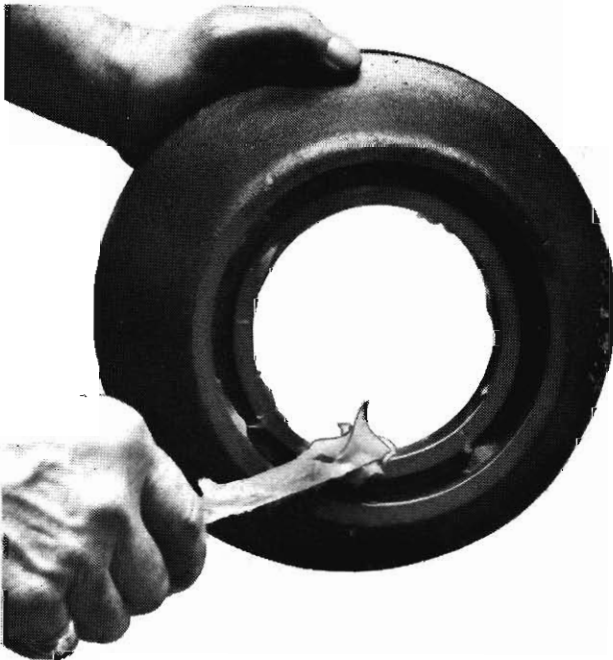
Fig. 1 - Grease Application To Labyrinth Grooves
