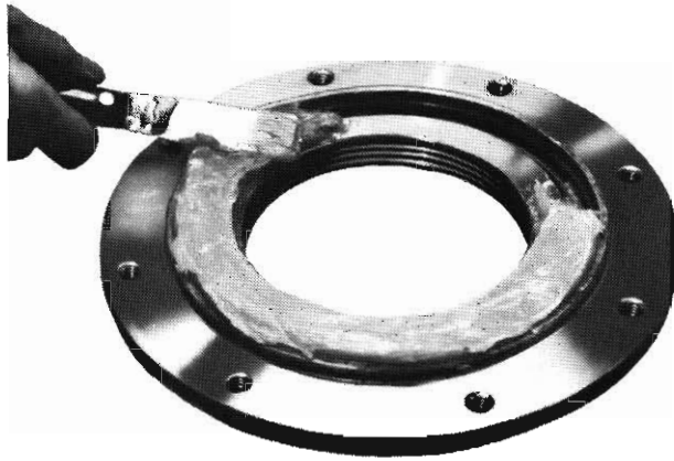
Fig. 3 - Roughly Formed Grease Contour
