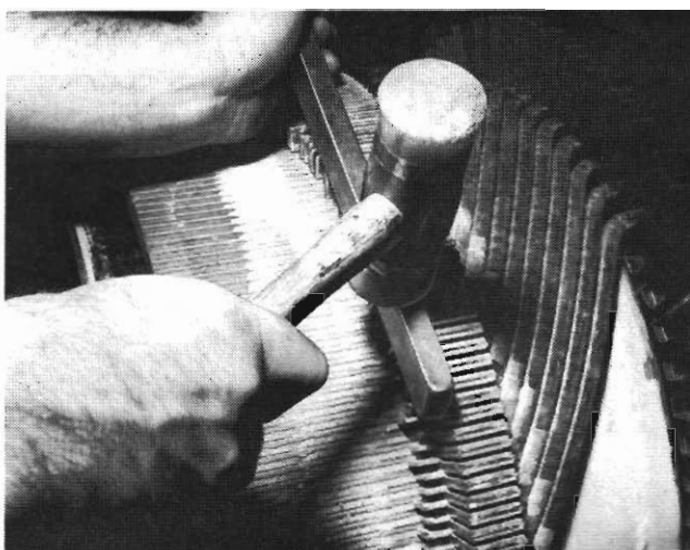
Fig. 38 - Temporarily Setting Coil Ends And Plugs In Riser
