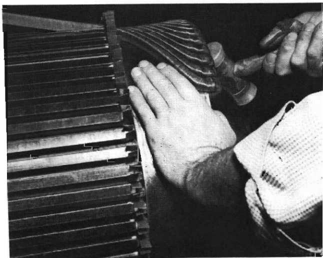
Fig. 43 - Shifting Coil Ends To Aid Pad Insertion
