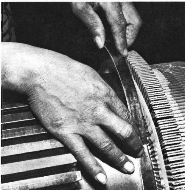
Fig. 22 - Installing Formed Mica Ring Behind Riser
