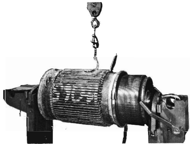
Fig. 3 - Removing Armature Coils
