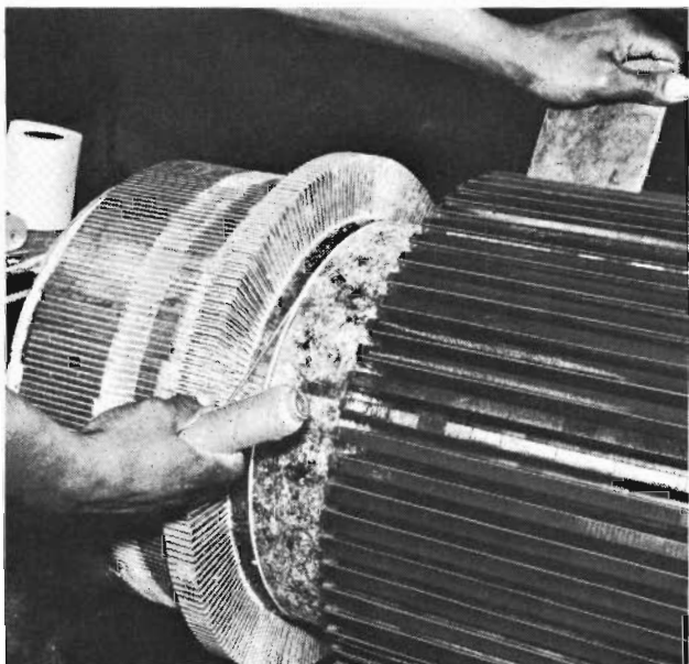
Fig. 33 - Filling In Gap Between Insulation
