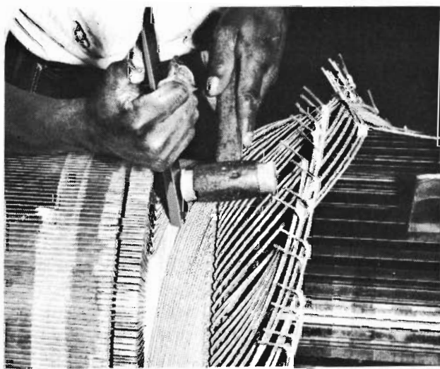
Fig. 41 - Drifting Connectors Into Position
