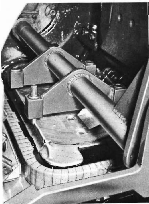
Fig. 18 - Aligning Fixture In Position
