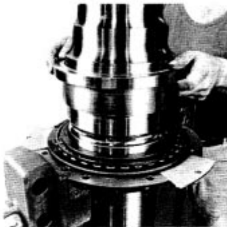
Step 23 Seat bearing inner race
