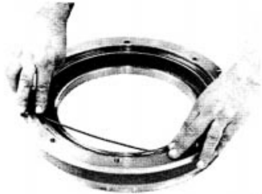
Step 26 O-ring seal to bearing cap
