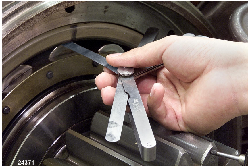
Figure 13 Using Feeler Gauge to Check Clearance
