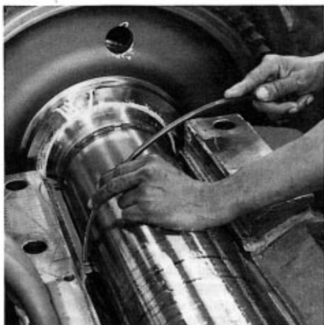
Fig. 3 - Threading Seal Ring Into Bearing Circumferential Groove
