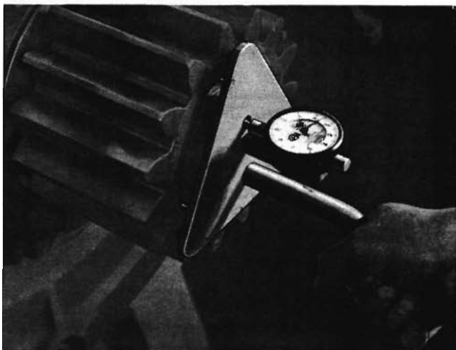
Fig. 24 – Measuring Pinion Advance
