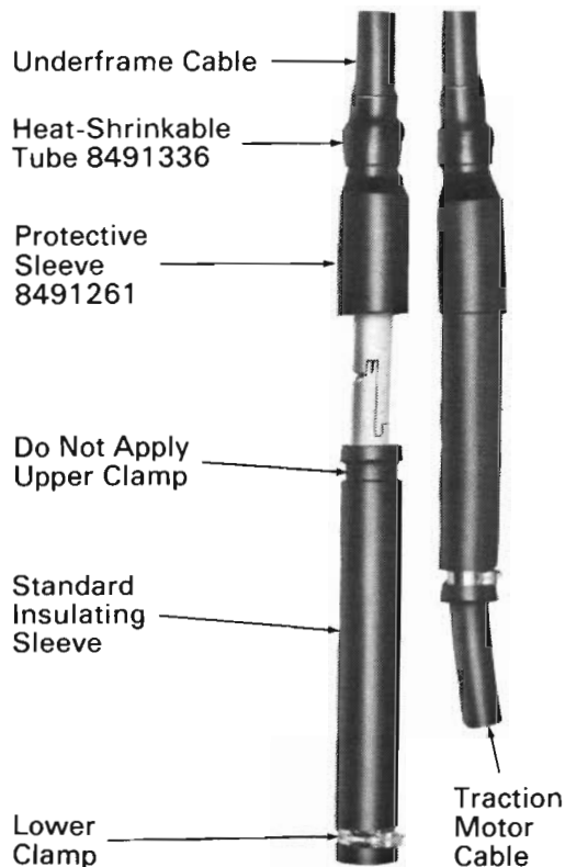
Fig. 62 – Protective Sleeve Applied To Traction Motor Clasp Connector
