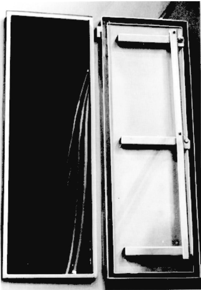
Fig. 32 - Sponge Rubber Tape Applied To Interior Perimeter Of Inertial Filter Compartment-To-Generator Personnel Door
