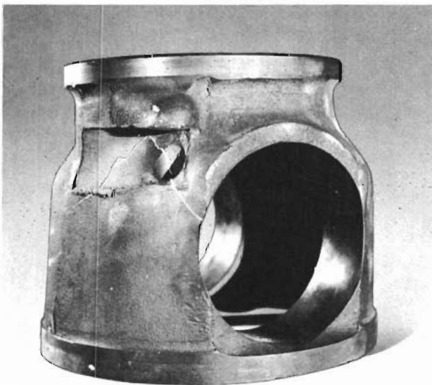
Fig. 23 - Defect Progression From Oil Hole
