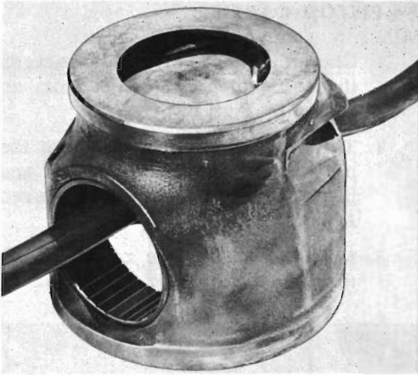
Fig. 19 - Magnetizing With Single Cable
