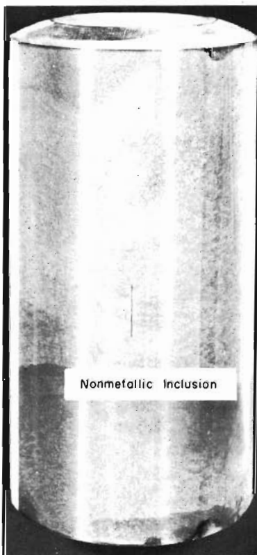
Fig. 30 - Nonmetallic Inclusion Indications
