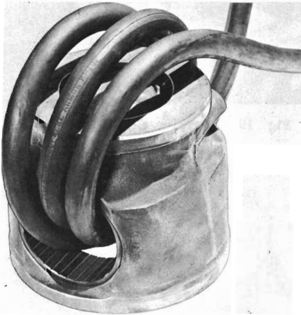
Fig. 20 - Magnetizing With Multiple Cable
