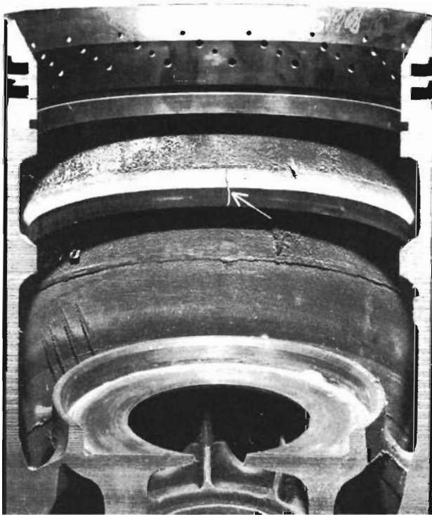
Fig. 16 - Pin Ring Magnaflux Indication
