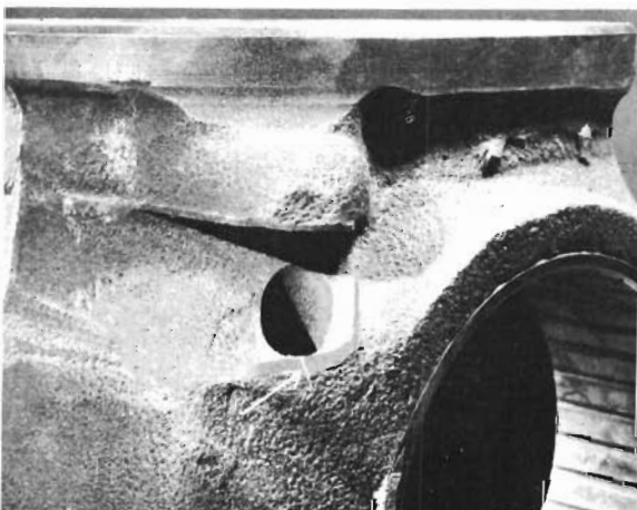
Fig. 21 - Oil Hole Defect Indication
