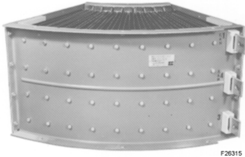
Figure 16 Dynamic Brake Grid Resistor With Control Tap
