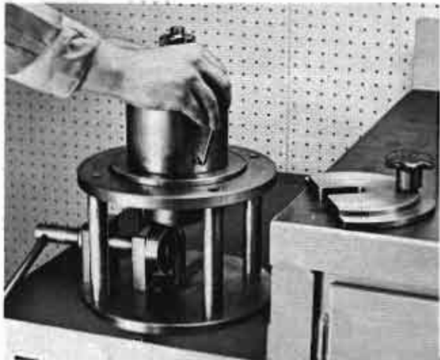
Fig.35 - Application Of Adapter Sleeve
