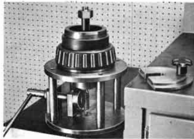
Fig.36 - Application Of Cone Assembly And Cone Spacer On Adapter Sleeve
