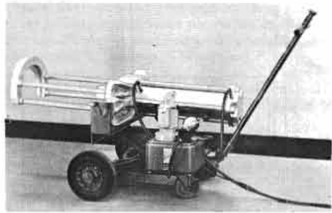
Fig.58 - Bearing Removal/Installation Fixture With Electrically-Operated Pump
