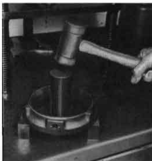
Fig.33 - Alternate Method Of Removing Seal Wear Ring
