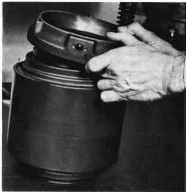
Fig.49 - Positioning Backing Ring
