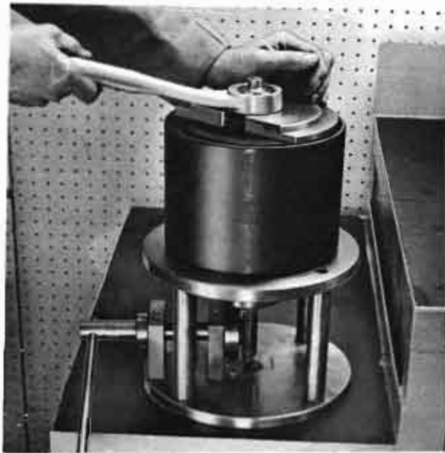
Fig.37 - Clamping Cone Assemblies And Cone Spacer
