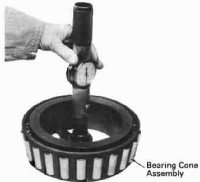
Fig.23 - Checking Cone Bore With Dial Bore Gauge
