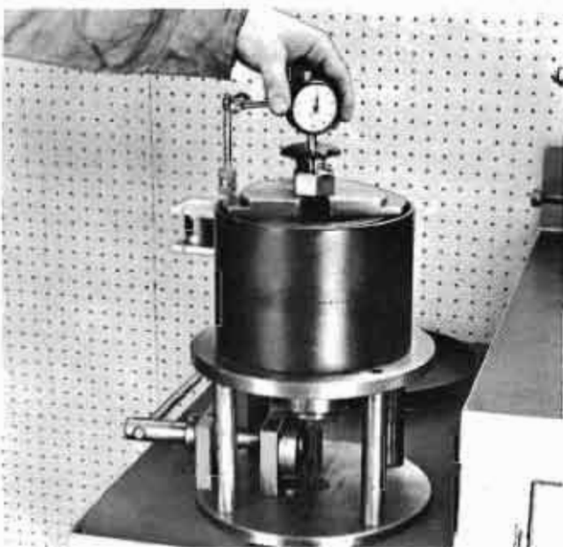
Fig.39 - Application Of Dial Indicator
