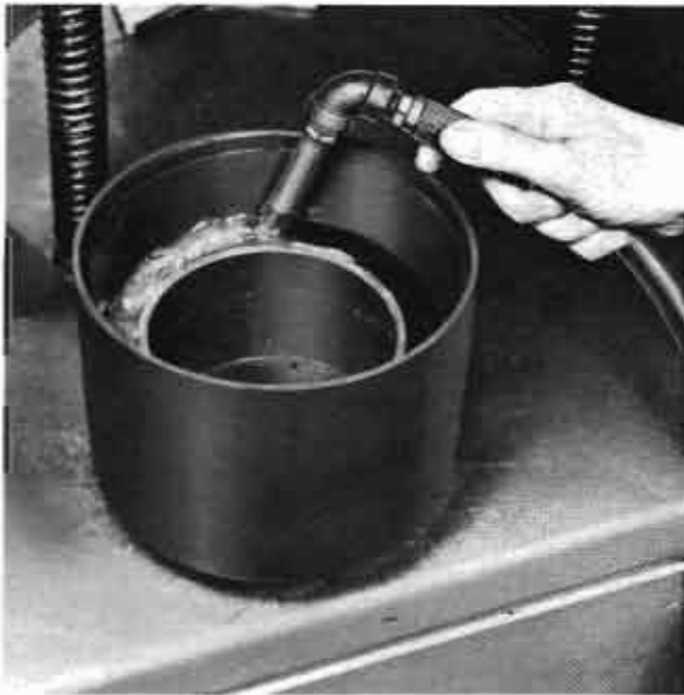
Fig.48 - Applying Grease Around Cone Spacer
