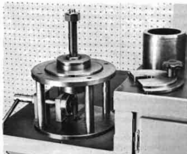
Fig.34 - Device For Checking Bearing Bench Lateral Play
