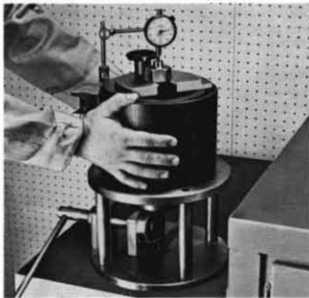
Fig.40 - Seating Lower Cone Assembly Rollers
