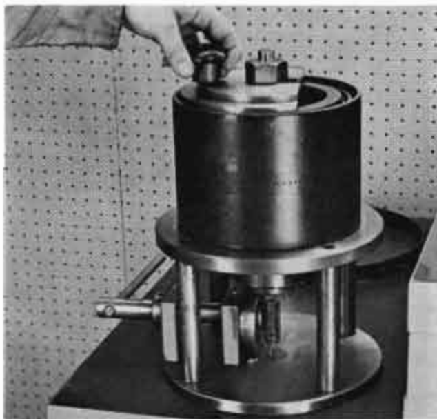
Fig.38 - Seating Upper Cone Assembly Rollers
