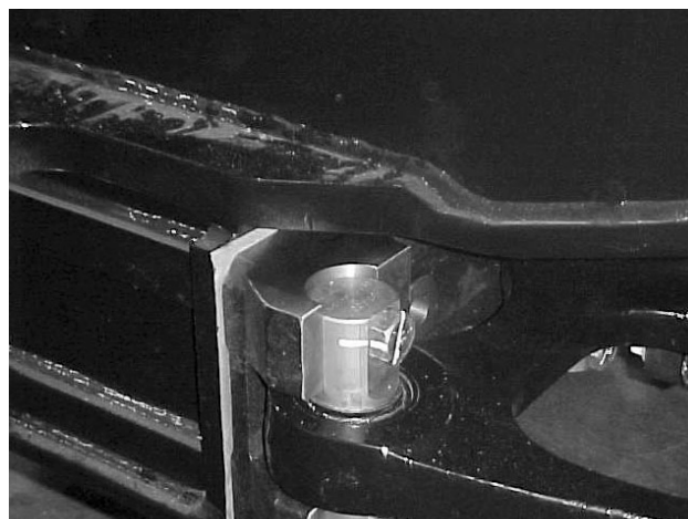
Figure 28 Tie Rod Bushing Mounting Bolt Showing Torque Line
