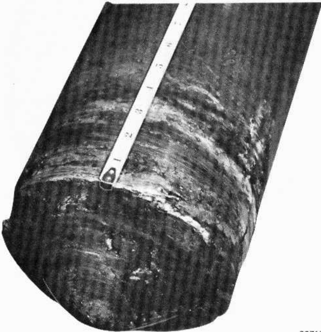
Fig.18 - Support Bearing Failure Due To Lack Of Lubrication
