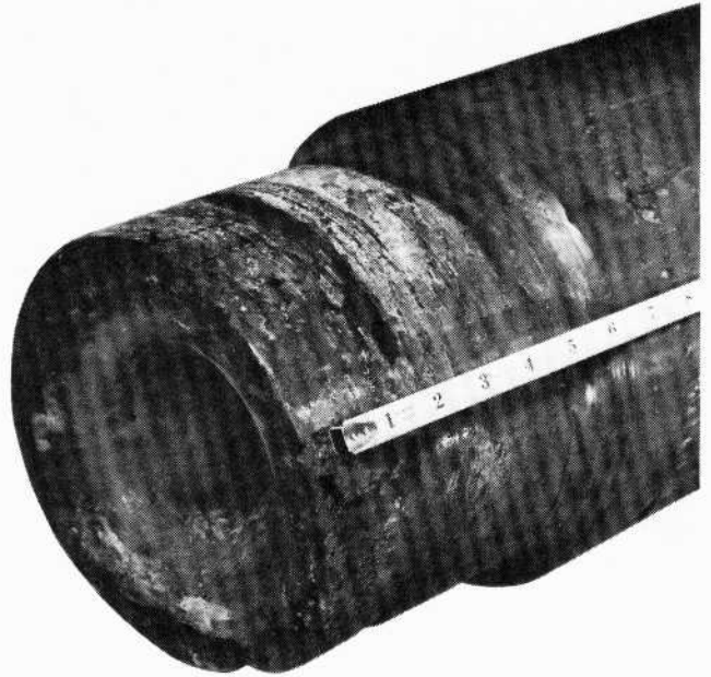
Fig.18 - Support Bearing Failure Due To Lack Of Lubrication
