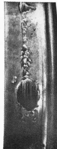
Fig. 15 -- Built-Up Tread And Slid Flat
