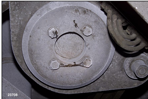
Figure 27 – Lock Wire and Bolt Removal
