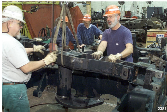
Figure 50 – Steering Beam Removal
