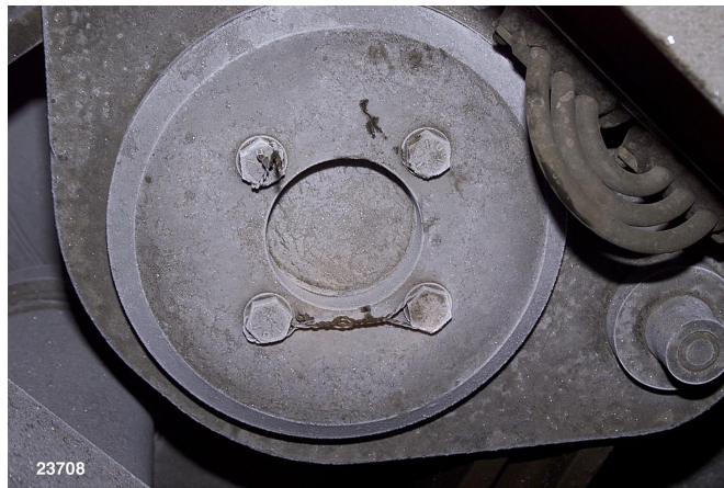
Figure 86 – Carbody Pivot Pin Lock Wire
