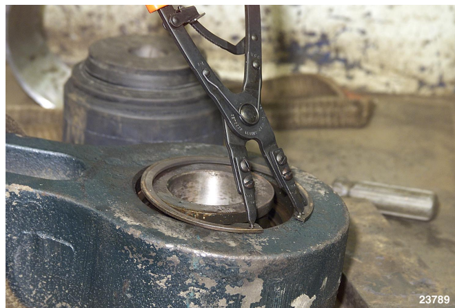
Figure 61 – Carbody Rod Snap Ring Removal
