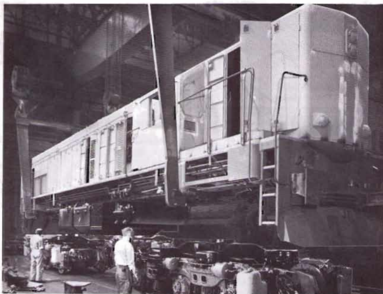
Fig. 3 - Locomotive Being Lifted From Trucks
